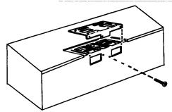
4. Remove and save the screw that holds blower motor to microwave.
